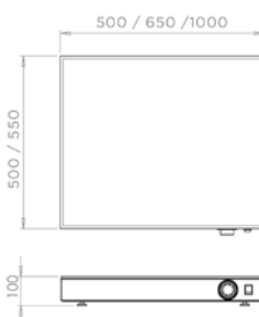
TEMPERED GLASS HOT PLATE COUNTERTOP DIMENSIONS
